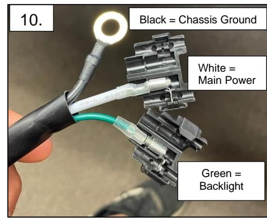
11. Remove the splice connector from the green wire.
