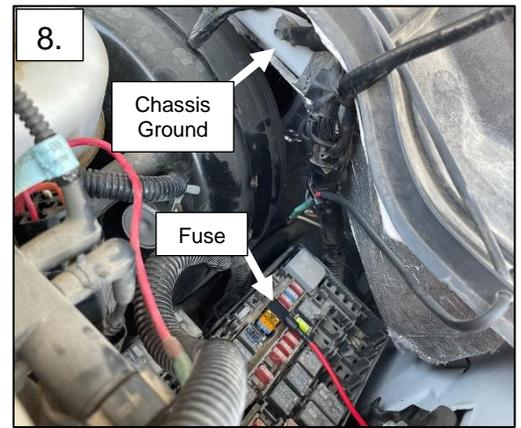
9. Remove the fuse box lid and the 15 amp fuse from slot 33 (Vehicle Power). Refer to the lid for fuse locations. Place the 15 amp fuse into the fuse tap shown.
